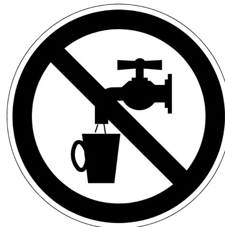
Diagram 10 Signage for non-potable water (Par. 1.3.10.2)
