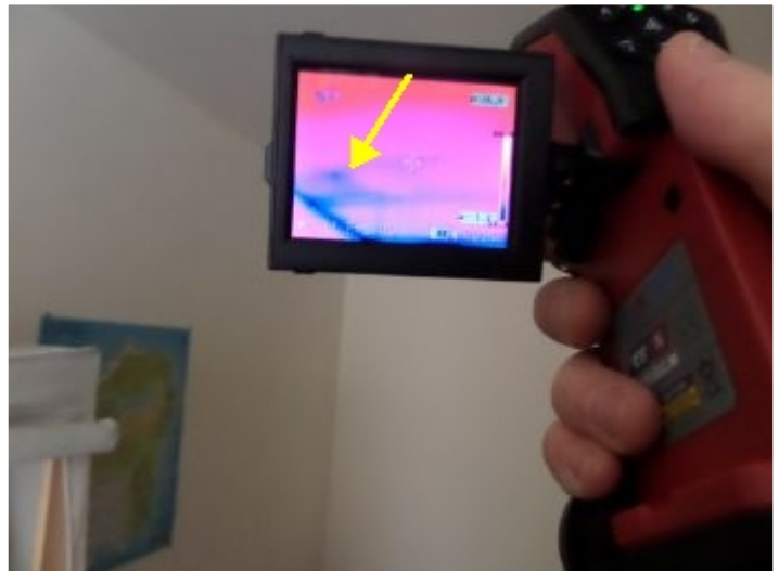
Sections of insulation missing / poorly fitted on attic floor.
