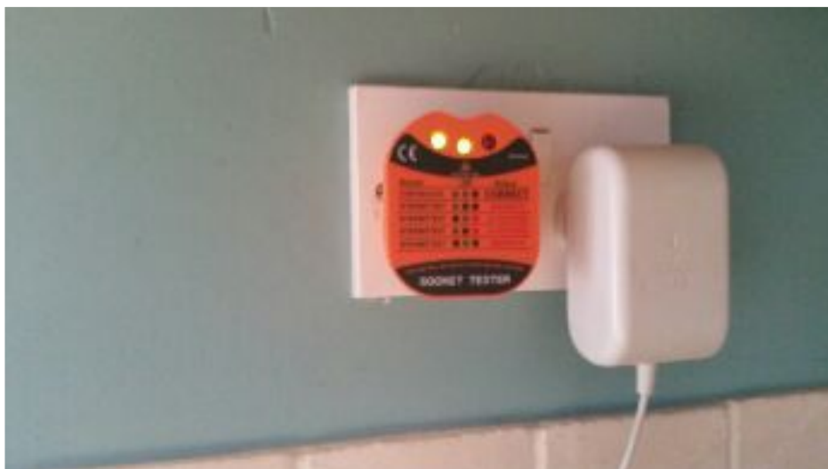
Wiring to plug sockets is earthed.
